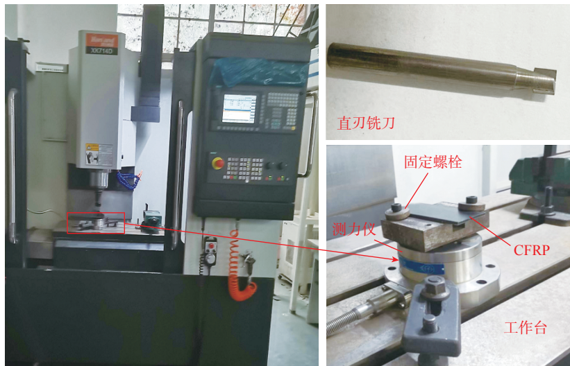
图4 单向CFRP切削试验装置 Fig.4 Unidirectional CFRP cutting test device
